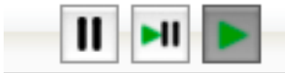
Figure 4: To change from continuous acquisition mode to single shot mode push the center button. Each time you push the center button a new exposure is recorded in memory. To return to continuous acquisition mode push the right hand button. To pause, push the left button. Save your spectrum by clicking the floppy disk icon on the menu bar above the spectrum.
