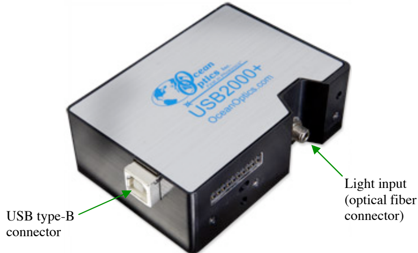
Figure 1: The Ocean Optics USB 2000 spectrometer. The spectrometer entrance slit is located at the rear of the SMA 905 type threaded connector. Commands to expose the CCD are sent via a USB connection and the data are returned via the same route.
